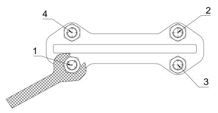
Figure 5: Tighten gland nuts crosswise
